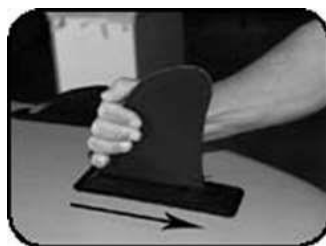
Slide fin all the way to back of fin box
