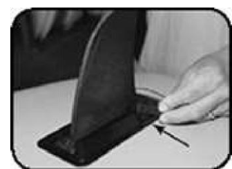
Insert fin clamp pin through the slot
